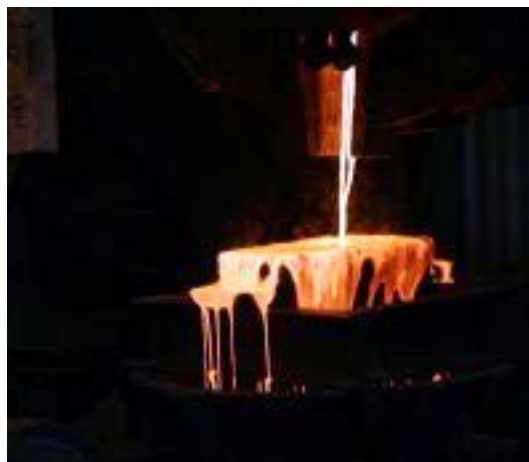
Figure 1 - Gold Pour, Rock Creek Mine, Nome, Alaska Source: NovaGold
